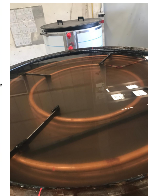
PCM heat exchanger, Paksoy, 2025
