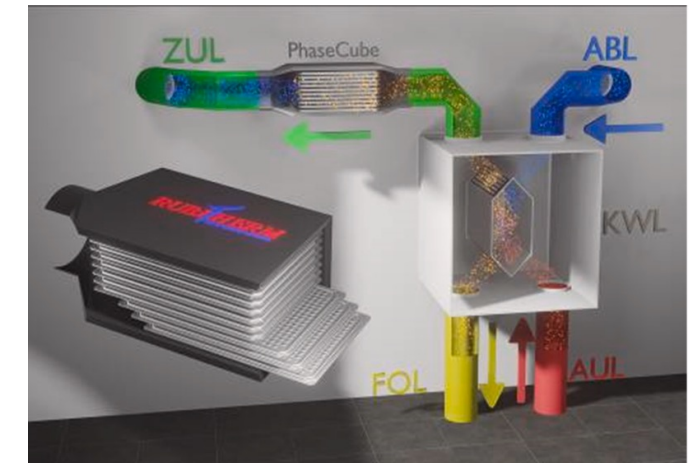
PCM plates in air ducts, Mehling, 2022
