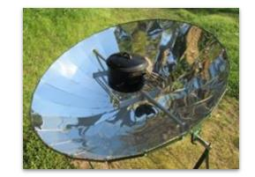
Reflective surfaces should be kept clean using only water and a clean rag
